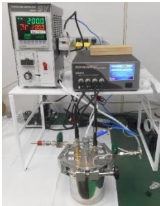
Fig.1 The AC impedance measurement system (NEISYS, 22cm-coaxial cables and the fixture).
