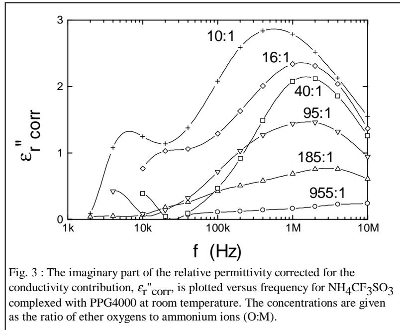
Fig. 3 : The imaginary part of the relative permittivity corrected for the conductivity contribution,  $\epsilon_r'' \text{corr}$ , is plotted versus frequency for  $\text{NH}_4\text{CF}_3\text{SO}_3$  complexed with PPG4000 at room temperature. The concentrations are given as the ratio of ether oxygens to ammonium ions (O:M).
