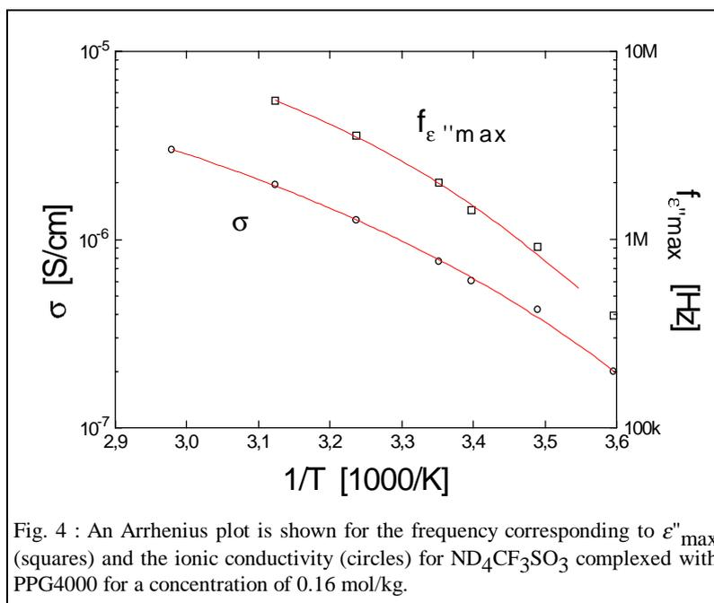
Fig. 4 : An Arrhenius plot is shown for the frequency corresponding to  $\epsilon_r'' \text{max}$  (squares) and the ionic conductivity (circles) for  $\text{ND}_4\text{CF}_3\text{SO}_3$  complexed with PPG4000 for a concentration of 0.16 mol/kg.
