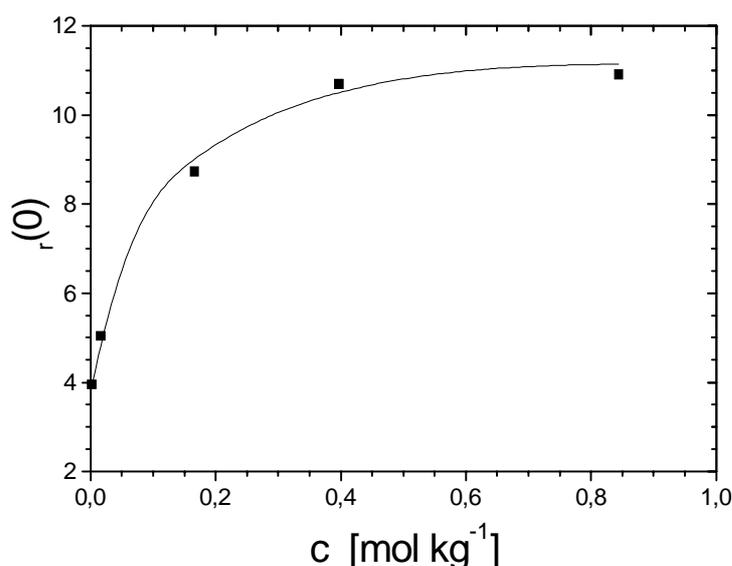
Fig. 2 : The static permittivity of  $\text{AgCF}_3\text{SO}_3$  dissolved in PPG4000.
