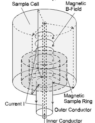
Fig. 1 : Principle of the sample cell for magnetic material measurements.
