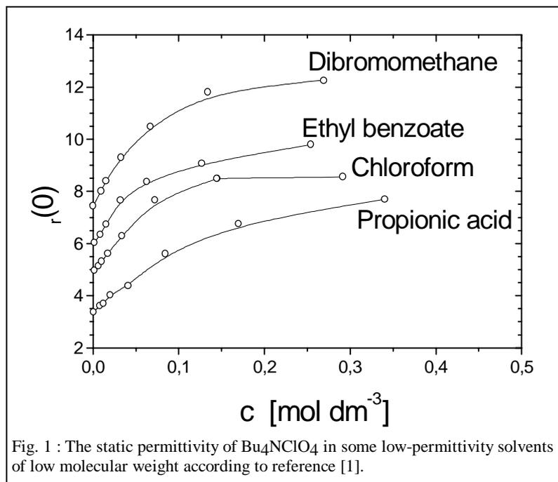
Fig. 1 : The static permittivity of  $\text{Bu}_4\text{NClO}_4$  in some low-permittivity solvents of low molecular weight according to reference [1].
