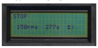
During operation, a built-in digital LC display with 20 characters per line informs about the rotation speed and the remaining ramp or dwell times for testing under reproducible conditions. It also substantially facilititates the set-up of the spin coater. For the sake of reproducibility, the set-up is stored permanently in the SCE-150 nonvolatile memory.
