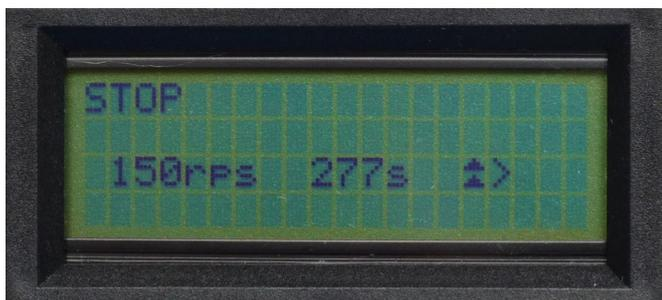
During operation, a built-in digital LC display with 20 characters per line informs about the rotation speed and the remaining ramp or dwell times for testing under reproducible conditions. It also substantially facilitates the set-up of the spin coater. For the sake of reproducibility, the set-up is stored permanently in the SCE-150 non-volatile memory.
