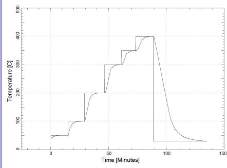
Stabilization characteristics of the sample temperature (process value) in dependence of the temperature set point. Set point step after sample temperature stabilization.
